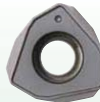
12mm iC Insert WOEJ1207 Up to .078" Ap max Diameter range 1.5–5"
